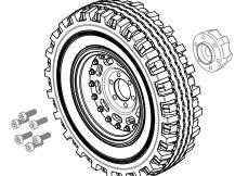
Remove the XT6 wheel hub from its original position as a single rear wheel.
